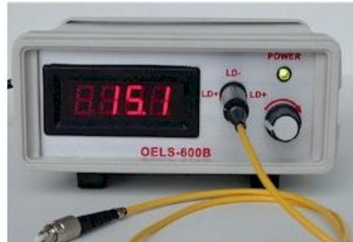
Fig.2 Laser Diode Driver System with Fiber Coupled Laser diode
