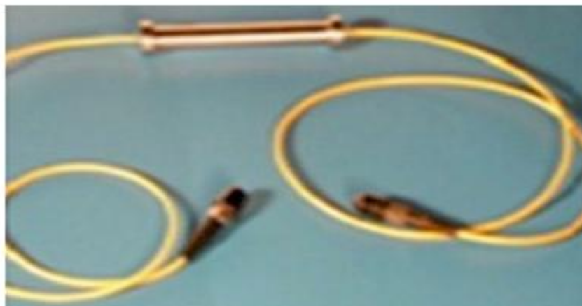
Figure 4: FBG Strain Sensor with embedded mount
